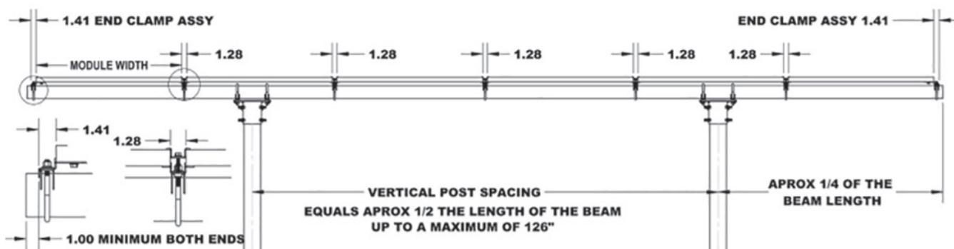
When using a single vertical pole (4" Sch-40 pipe) (1-4 modules) center the beam over the vertical post.
