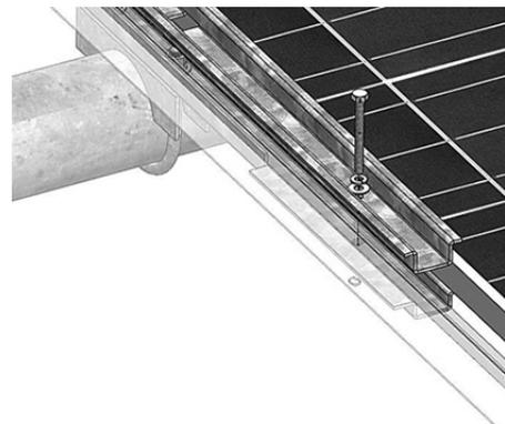
Install Mid Clamp tops with the 1/4 x 2.5-inch hex bolts, flat & lock washers after the mid clamps have been moved tight against the module frames.
